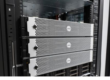
Enhance your site security and improve incident response times with the **Avigilon Al Appliance**, enabling advanced video analytics on existing cameras. The **Al Appliance** addresses critical security gaps without costly hardware replacements, supports up to 160 cameras and delivers Server-side Analytics. Future-proof your security infrastructure with the **Al Appliance 2X CG3** model, which leverages the latest advancements in Generative Al for improved situational awareness.
